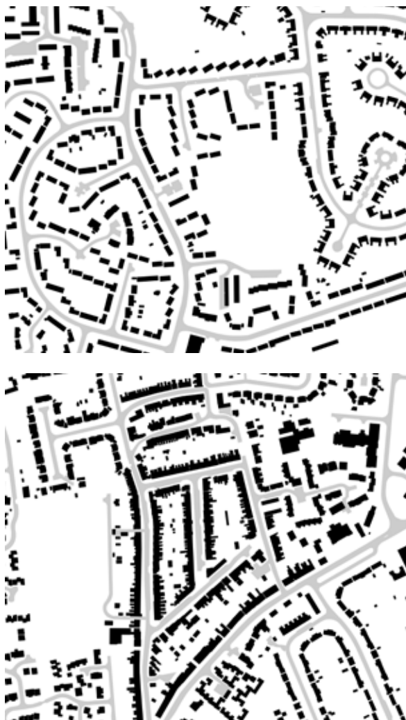
Figure 4.3 Inappropriate dispersed, cul-de-sac and car-dependent layout (top) versus traditional, connected, walkable layout (bottom). Both examples from Banbury
